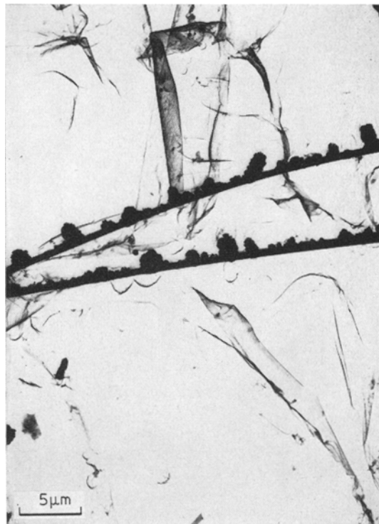
Figure 4 Irregular nickel particles on CTH whiskers after 17 h at 1200°C (initial coating 80 nm).
